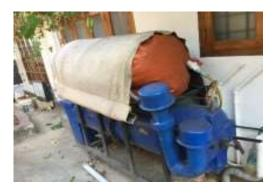
As part of the program, we have installed around 20 Biogas units in the program area. A digester of 350-litre volume is sufficient to treat around 3 kilograms wastes a day. It produces 250 to 600 liters of methane-rich biogas daily by loading of 1 to 3 kg wastes as input.
